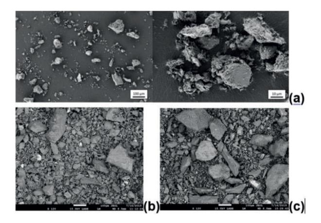
Scanning electron microscopic close-ups of simulated lunar regolith, showing (a)
