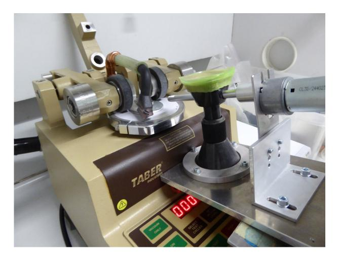
Rotary Platform Double Head Abraser with lunar soil simulant. The simulant is fed continuously to the abraser platform to account for new portions of lunar dust in contact with the suit's external layers. The tested materials are further investigated in terms of weight and microscopic image. Credit: DITF
