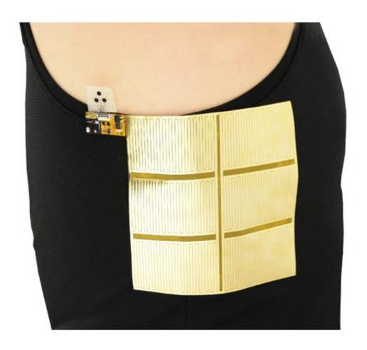
Wei Gao's triboelectric generator is made of commonly available commercial materials and creates electricity when the wearer moves. Credit: Caltech
