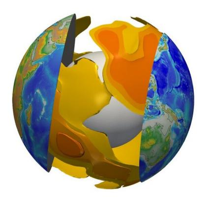
Three-dimensional visualisation of partial melting at the base of tectonic plates. The orange iso-surfaces show the regions where, at a depth of between 100 and 300 km, the quantity of molten rock is greater than 0.2%. The white sphere in the centre of the globe represents the Earth's core. Credit: Stéphanie Durand, Laboratoire de géologie de Lyon: Terre, planètes et environnement (CNRS/ENS de Lyon/Université Claude Bernard Lyon 1).
