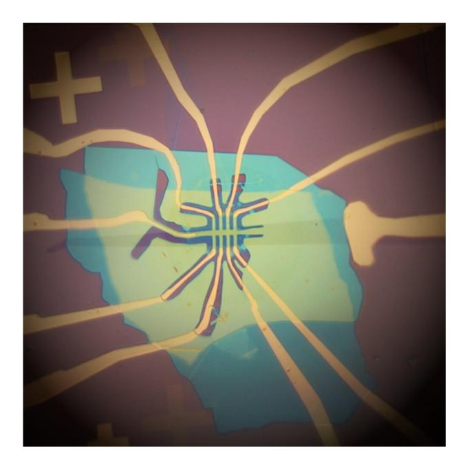
Optical microscopy image of a twisted double bilayer graphene device. Credit: Matthew Yankowitz
