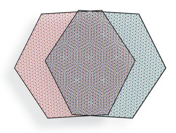
Illustration of a moiré pattern that emerges upon stacking and rotating two sheets of bilayer graphene. Correlated electronic states with magnetic ordering emerge in twisted double bilayer graphene over a small range of twist angles, and can be tuned with gating and electric field. Credit: Matthew Yankowitz
