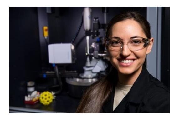
PNNL chemist Jordan Corbey and the single-crystal X-ray diffractometer. The instrument uses X-rays to determine the identity of each atom and draw a map of how they bond to each other. Credit: Andrea Starr | PNNL
