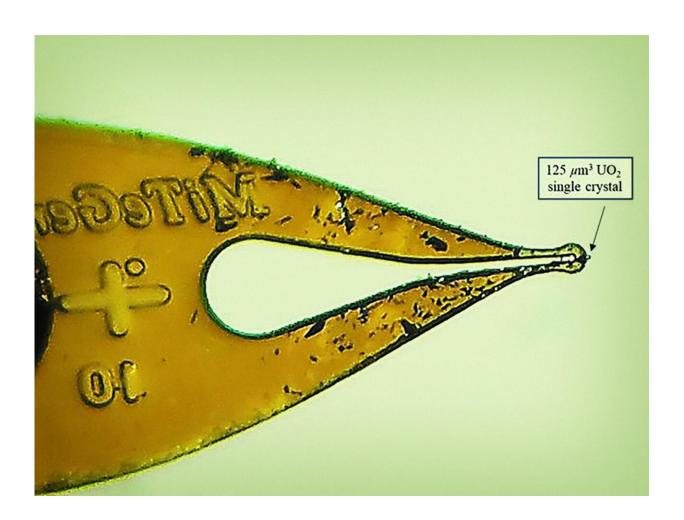
Optical microscope image of a single radioactive microcrystal. Credit: Jordan Corbey | PNNL
