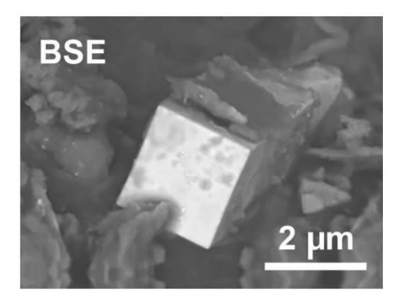
A single plutonium crystal from Hanford trench soil. This crystal is twenty times smaller than a grain of table salt. Credit: Jordan Corbey | PNNL
