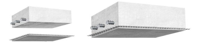
(Left) Deteriorated concrete member and precast TRM panel; and (Right) Concrete member strengthened with TRM panel. Credit: Korea Institute of Civil Engineering and Building Technology (KICT)
