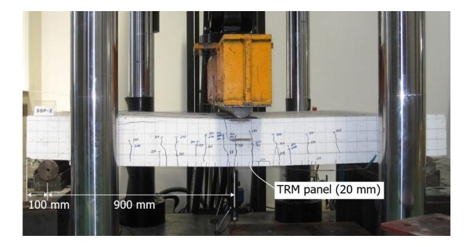
Failure test of a concrete slab strengthened with TRM panel. Credit: Korea Institute of Civil Engineering and Building Technology (KICT)
