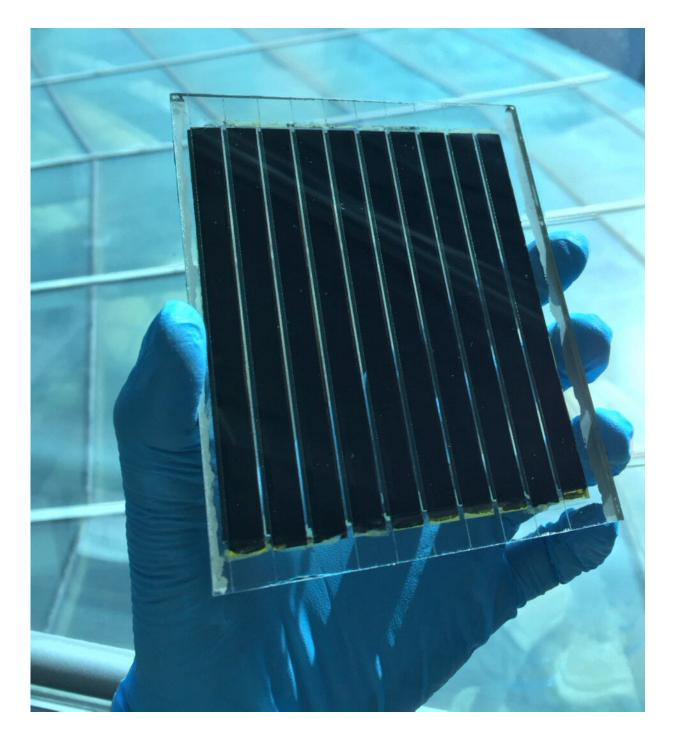
Publishing in *Science*, researchers at EPFL have successfully overcome a limiting problem with stabilizing the best-performing formulation of metal-halide perovskite films, a key player in a range of applications, including solar cells. Credit: Nripan Mathews NTU, Singapore
