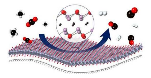
A thin film of metal oxycarbides on an oxide support facilitates the reaction between  $CO_2$  and methane (CH4) to produce hydrogen (H2) and carbon monoxide (CO). Credit: Alexey Kurlov, Evgenia Deeva / ETH Zurich
