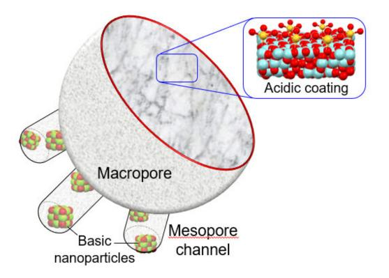
A graphic illustration showing how the catalyst performs several chemical reactions in sequence within a single catalyst particle, with molecules entering the sponge through the large pores (macropore) then passing into smaller pores (mesopore). Credit: RMIT University
