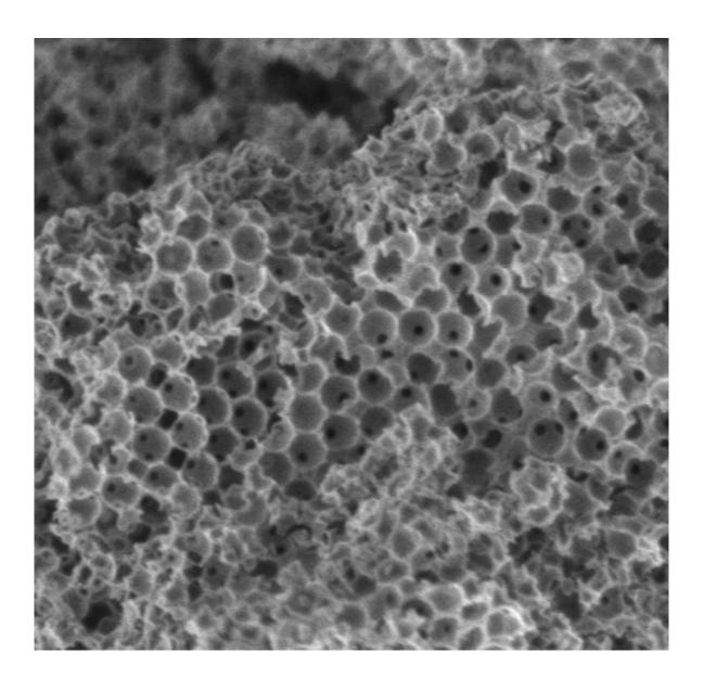
Sponge-like catalysts could transform biodiesel production and chemical manufacturing. Image shows the porous ceramic sponge fabricated in the study (magnified 20,000 times). Credit: RMIT University
