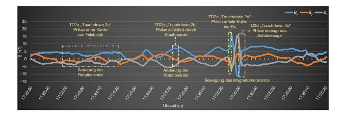
Philae's magnetometer measurements on TD2. Credit: ESA/Rosetta/Philae/ROMAP
