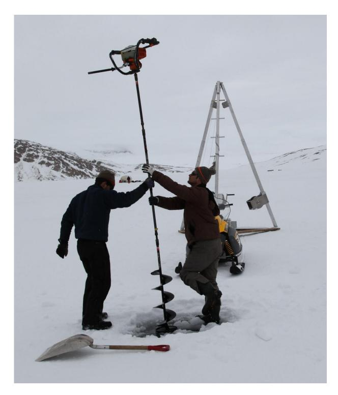
Climate scientists Nicholas Balascio and Francois Lapointe working with an ice auger to drill in the 3.5m thick ice at South Sawtooth Lake, Ellesmere Island, Nunavut Territory, Canada. An ice auger extension is needed because the ice is so thick. Coring lake sediments can only be done after this tedious work,
