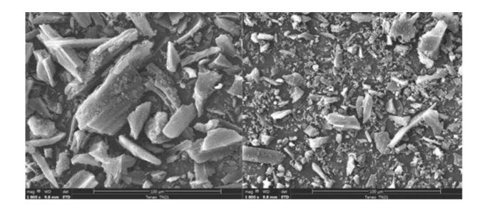
SEM photo of (left) existing powder activated carbon and (right) powder activated carbon developed by KIST researchers by grinding it using ball mil Credit: Korea Institue of Science and Technology(KIST)
