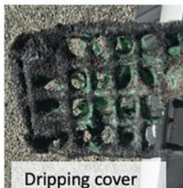
Melted meters under glass covers
