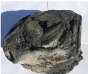
Misshapen melted meter
