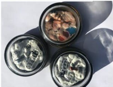
Melted meters under glass covers
