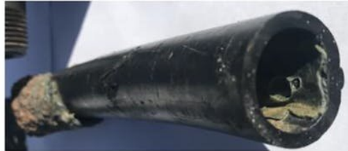
Whole view of pipe A with A melted plastic inside (A1) and melted plastic on outside (A2)
