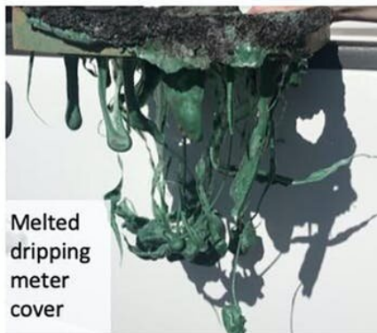
Water meter cover (green) that melted and fused to a meter and service line (brown/white/black)
