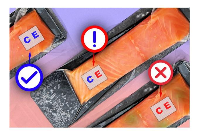
The researchers attached the sensor to a fillet of raw fish that they had injected with a solution contaminated with E. coli. After less than a day, they found that the part of the sensor that was printed with bacteria-sensing bioink turned from blue to red — a clear sign that the fish was contaminated. After a few more hours, the pH-sensitive bioink also changed color, signaling that the fish had also spoiled. Credit: Jose-Luis Olivares, MIT. Sensor texture courtesy of the researchers
