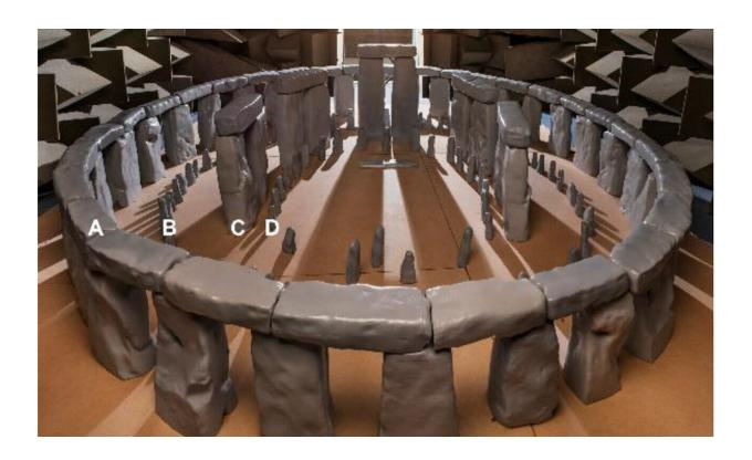
The 1:12 Acoustic Scale Model of Stonehenge in the semi-anechoic chamber. This is the monument after the bluestones had been re-arranged, c.2200 BC. It is approximately 2.5 m wide. Text annotations: (A) outer sarsen circle; (B) outer bluestone circle; (C) inner trilithon horseshoe and (D) inner bluestone oval. Credit: *Journal of Archaeological Science* (2020). DOI: 10.1016/j.jas.2020.105218
