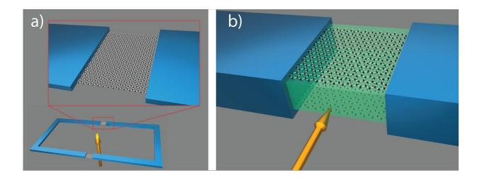
(a) A conventional superconducting quantum interference device (SQUID) consists of a superconducting ring interrupted at two points by weak links (in this case a graphene layer). (b) The new SQUID is made up of a stack of two-dimensional materials, including two graphene layers separated by a thin film of boron nitride. (University of Basel, Department of Physic
