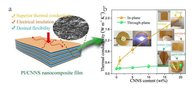
(a) The schematic diagram of PI/CNNS nanocomposite films; (b) the thermal conductivity and photographs of PI/CNNS nanocomposite films. Credit: WANG Yanyan
