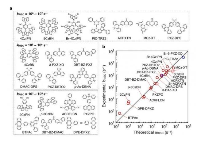
Figure 1. TADF materials examined in this study and their RISC rate constants (kRISC). a Molecular structures of the examined TADF materials categorized by their kRISC. b Comparison of the experimental and theoretical kRISC. Credit: Naoya Aizawa
