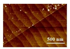
Figure shows (left) the concept of the terraced single-layer graphene formation. This is similar to the terraced paddy fields used widely in Asia for agriculture. (Right) Atomic force microscopy image of the terraced morphology for graphene on strontium titanate (STO, top left) and bare STO substrate (bottom right). Credit: Advanced Materials
