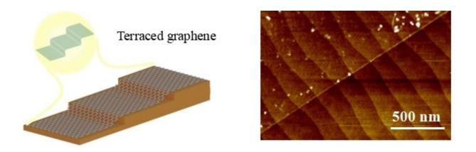
Figure shows (left) the concept of the terraced single-layer graphene formation. This is similar to the terraced paddy fields used widely in Asia for agriculture. (Right) Atomic force microscopy image of the terraced morphology for graphene on strontium titanate (STO, top left) and bare STO substrate (bottom right). Credit: Advanced Materials
