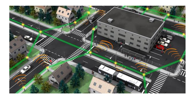
Future mobile network: Small radio cells (orange) are connected by wireless high-speed terahertz links (green). Credit: IPQ, KIT / *Nature Photonics*
