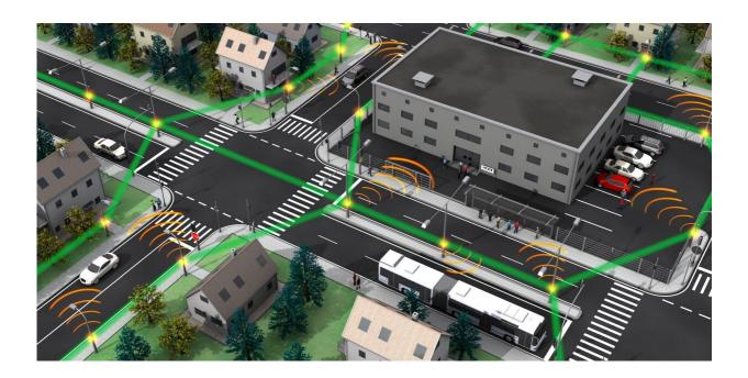
Future mobile network: Small radio cells (orange) are connected by wireless highspeed terahertz links (green). Credit: IPQ, KIT / *Nature Photonics*
