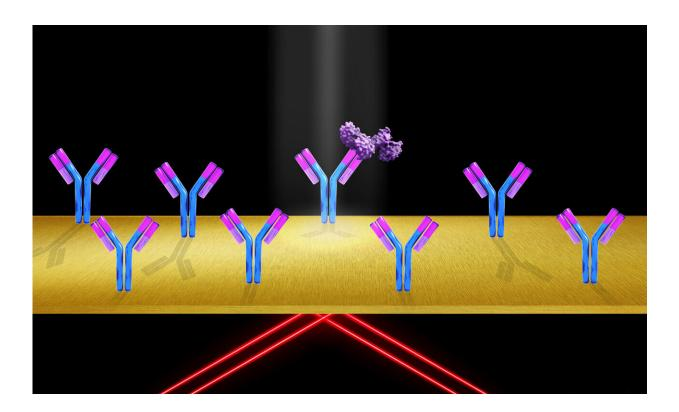
When protein molecules (purple) bind to immobilized receptor molecules, (like the Y-shaped antibodies affixed to the slide surface), the refractive index at the gold surface changes, altering the surface plasmon resonance condition, and producing an increase in signal intensity. Credit: Shireen Dooling
