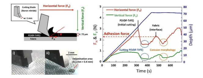
Measurement of an interfacial adhesion strength using SAICAS. Credit: KAIST
