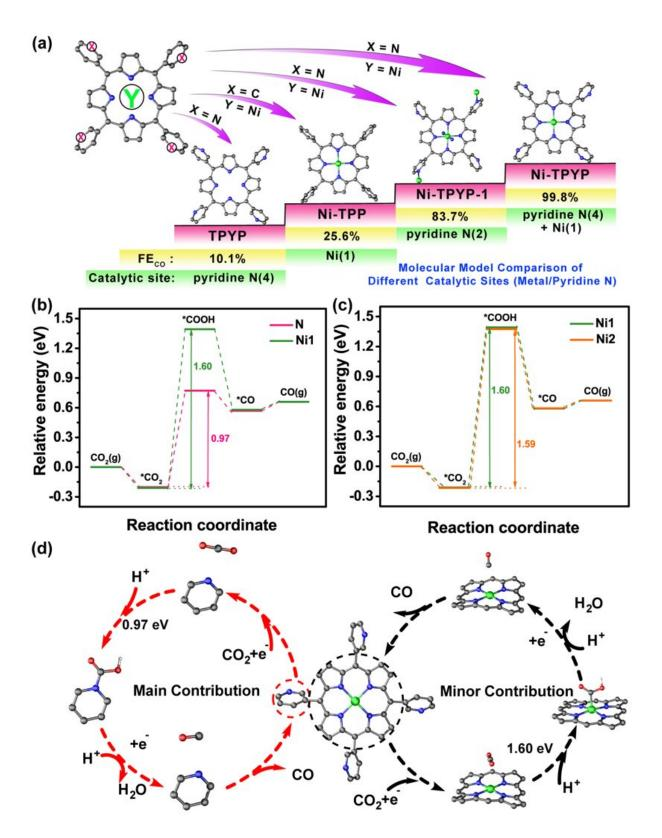
(a) Comparison of different molecular structures and catalytic sites (Ni-TPYP,
