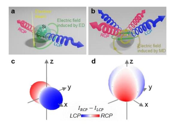
(a/c) Both left- and right-handed CPL are generated by the phase difference between two perpendicular electric dipoles, excited by the impact of the electron beam. (b/d) Left- and right-handed CPL is emitted at different angles because of the interference between electric dipoles and a magnetic dipole. Credit: ACS Nano
