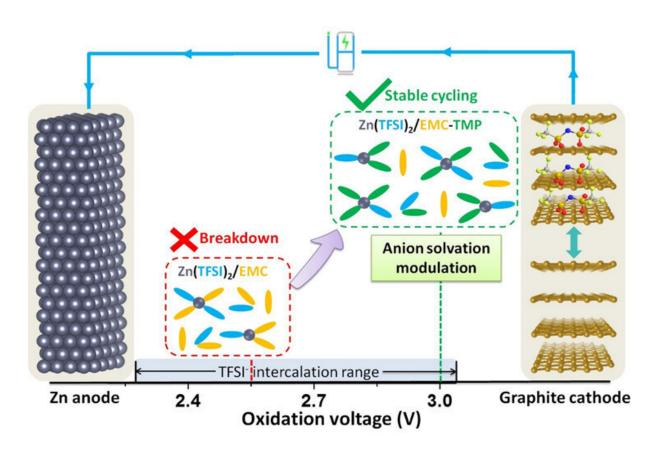
Tuning the anion solvation network of carbonate-based electrolyte for high-voltage Zn/graphite batteries. Credit: Zhao Jingwen
