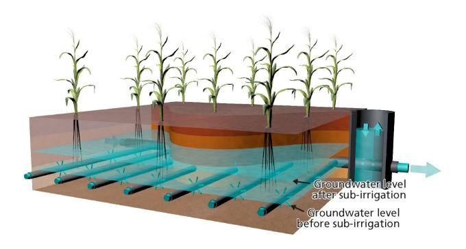
Schematic overview of sub-surface irrigation systems. Credit: Dominique M. Narain-Ford et al. 2020
