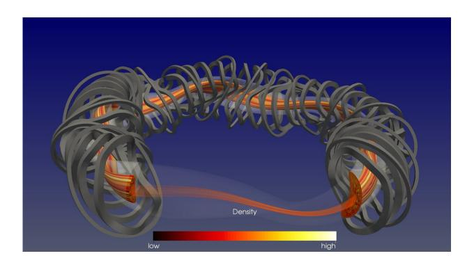
The magnetic cage generated by the magnetic coils (grey) shapes and encloses the plasma. The turbulent variation of the plasma density is to be seen in the plasma cross-section. Credit: IPP, A. Banon Navarro
