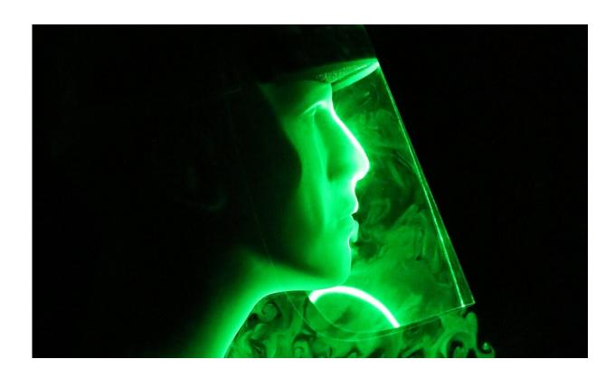
Although face shields block the initial forward motion of the jet, the expelled droplets move around the visor with relative ease and spread out over a large area depending on light ambient disturbances. Credit: Florida Atlantic University's College of Engineering and Computer Science
