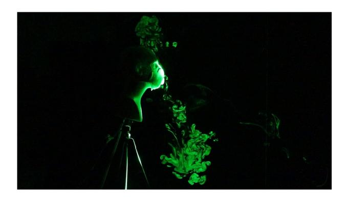
Researchers also tested an N-95 rated face mask with exhalation valves and found the exhalation port significantly reduced the effectiveness of the mask as a
