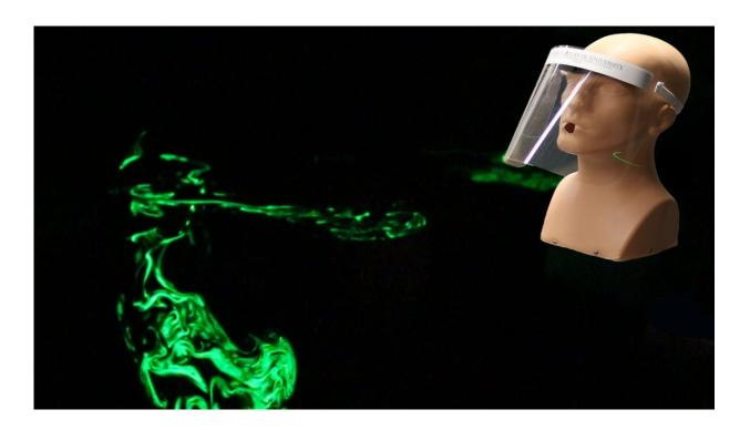
Far-field view of a droplet spread when a face shield is used to impede the jet,
