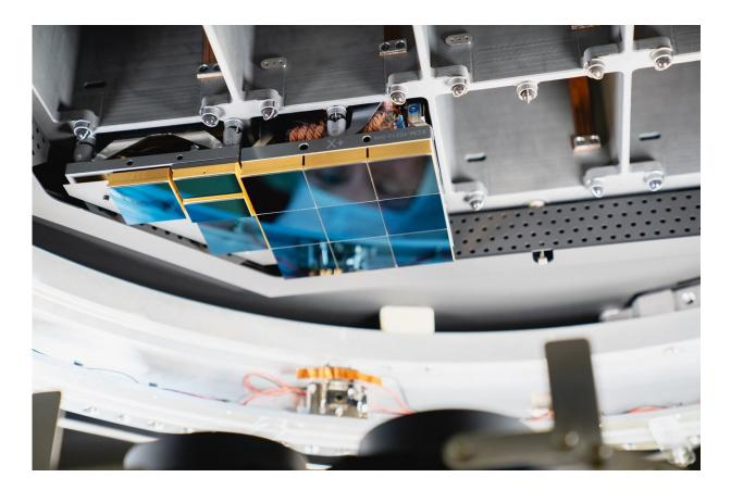
The complete focal plane of the future LSST Camera is more than 2 feet wide and contains 189 individual sensors that will produce 3,200-megapixel images. Credit: Jacqueline Orrell/SLAC National Accelerator Laboratory
