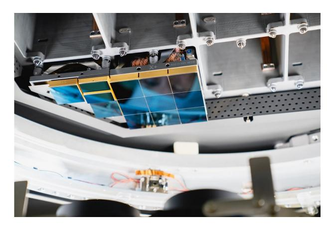
The complete focal plane of the future LSST Camera is more than 2 feet wide and contains 189 individual sensors that will produce 3,200-megapixel images. Credit: Jacqueline Orrell/SLAC National Accelerator Laboratory
