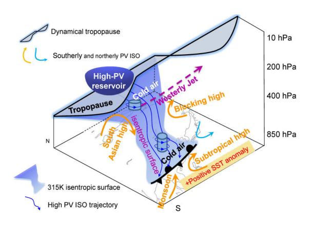
Schematic illustration of precursor signal and synoptic system configuration along isentropic surface for persistent strong precipitation events in South China. Credit: ZHAO Liang
