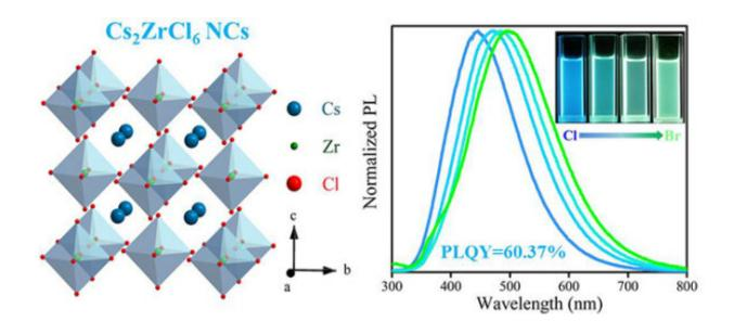
Lead-free perovskite Cs2ZrCl6 NCs with a PLQY up to 60.37% is synthesized. Credit: LIU Siping and YANG Bin
