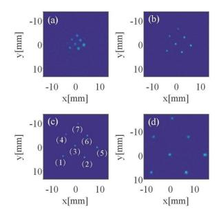
Beam images as a function of solenoid strength. Credit: Jiahang Shao / Argonne National Laboratory
