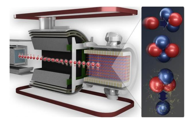
The n-helium-3 precision experiment, conducted at ORNL, measured the weak force between protons and neutrons by detecting the tiny electrical signal produced when a neutron and a helium-3 nucleus combine and then decay as they move through the helium gas target cell. Credit: Andy Sproles/ORNL, U.S. Dept. of Energy
