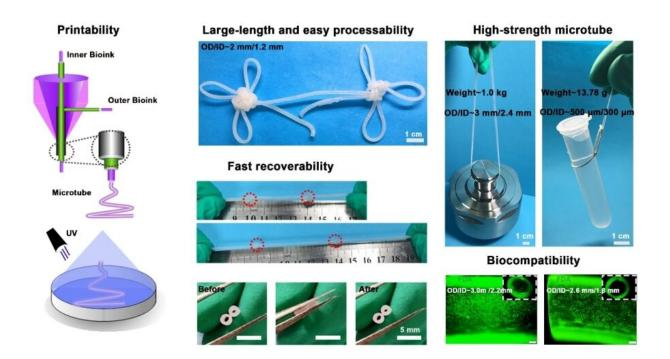
Schematic diagram of the fabrication and characterization of microtubes. Credit: SIAT
