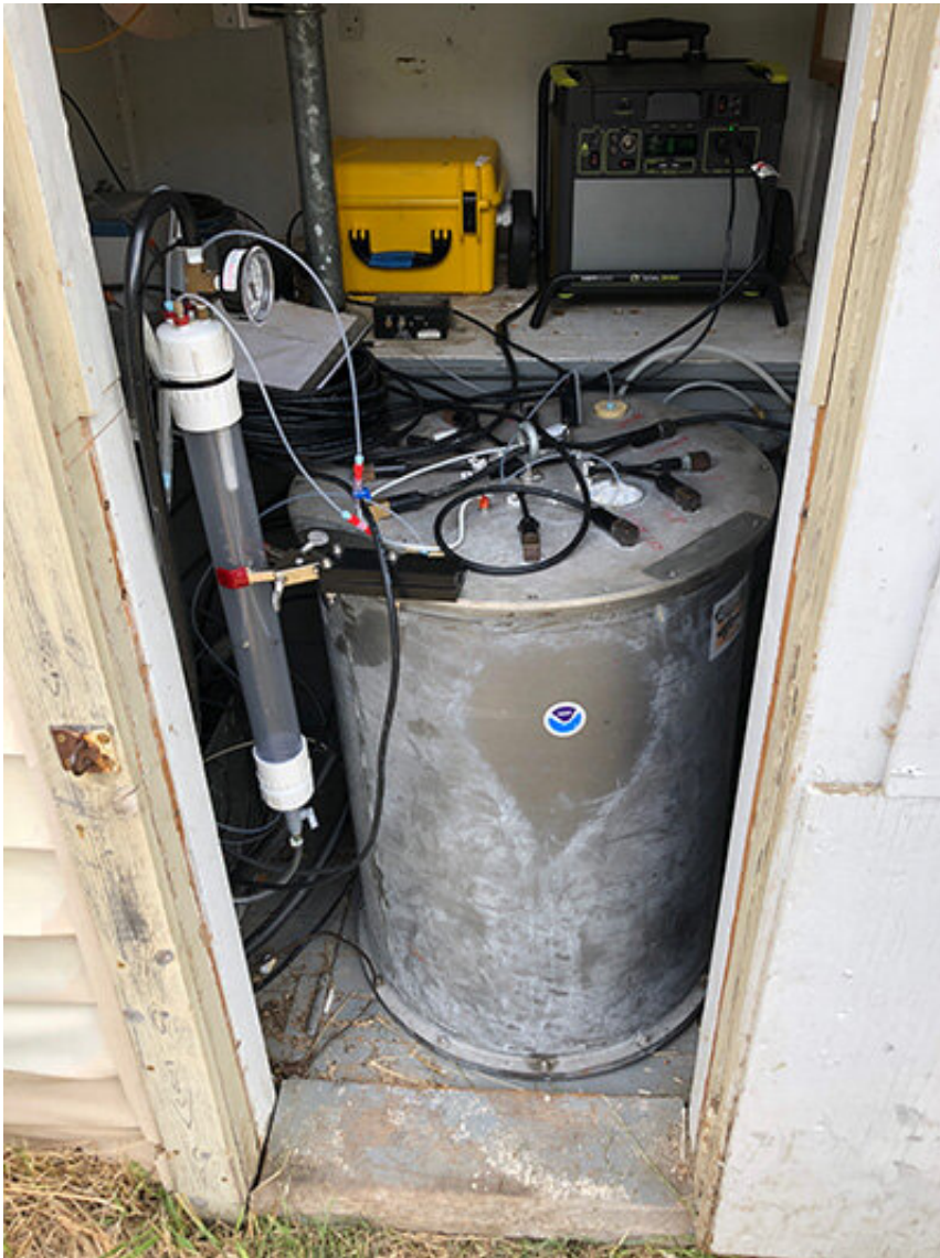
This photo shows an Environmental Sample Processor (large gray cylinder), along with filters and pumps inside a USGS streamgage station. Credit: Jim Birch/MBARI
