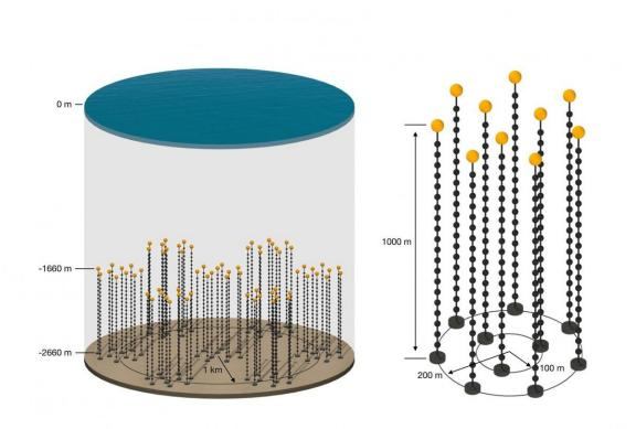
Design of the planned P-ONE neutrino telescope in the Pacific Ocean (left). The telescope will have a modular structure and consists of seven identical detector segments (right), the first of which will be installed in 2023/24. Credit: Elisa Resconi / TUM
