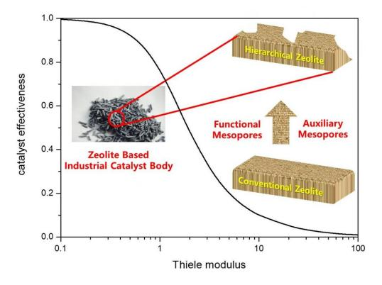
Hierarchical structures at both zeolitic component and industrial catalyst levels Credit: Science China Press
