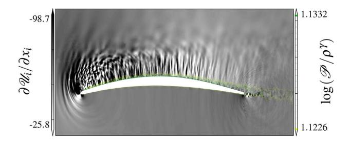
The researchers are modeling compressible airflows across surfaces under high turbulence to reveal the pressure waves we hear as sound. Credit: KAUST
