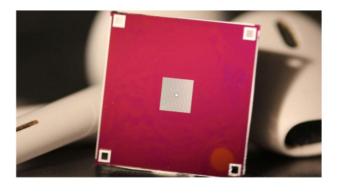
A thin silicon nitride membrane (white) is stretched tight across a silicon frame (red). The membrane contains a pattern of holes, with one small island in the center, whose vibrations are measured in the experiment. Credit: Niels Bohr Institute
