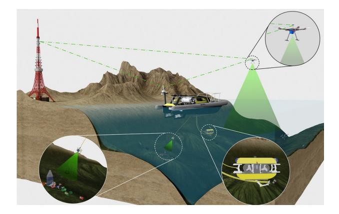
Various robot vehicles are networked with one another in the SeaClear system. An autonomous or remote-controlled mother ship (UPS) on the surface is supported by two underwater robots (ROV) and a flight drone (UAV). Credit: TUM
