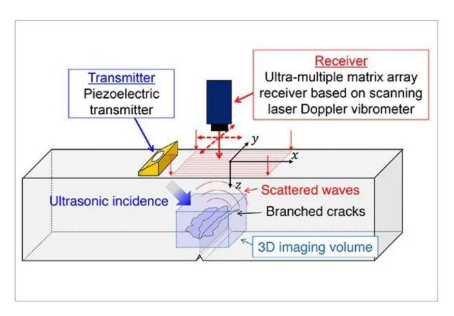
A Schematic illustration of the high-resolution 3D ultrasonic imaging system (PLUS). Credit: Yoshikazu Ohara, Tohoku University
