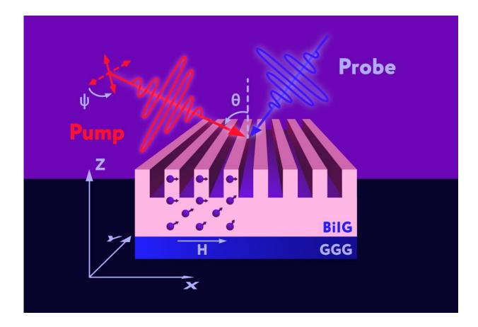
Schematic representation of spin wave excitation by optical pulses. The laser pump pulse generates magnons by locally disrupting the ordering of spins shown as violet arrows — in bismuth iron garnet (BiIG). A probe pulse is then used to recover information about the excited magnons. GGG denotes gadolinium gallium garnet, which serves as the substrate Credit: Alexander Chernov et al./Nano Letters
