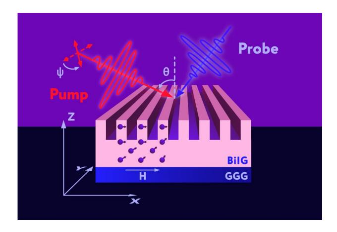
Schematic representation of spin wave excitation by optical pulses. The laser pump pulse generates magnons by locally disrupting the ordering of spins — shown as violet arrows — in bismuth iron garnet (BiIG). A probe pulse is then used to recover information about the excited magnons. GGG denotes gadolinium gallium garnet, which serves as the substrate Credit: Alexander Chernov et al./Nano Letters
