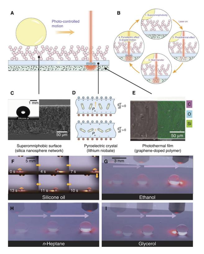
Design of photopyroelectric microfluidics. (A) Schematic of the trilayered photopyroelectric platform consisting of the superomniphobic surface (silica
