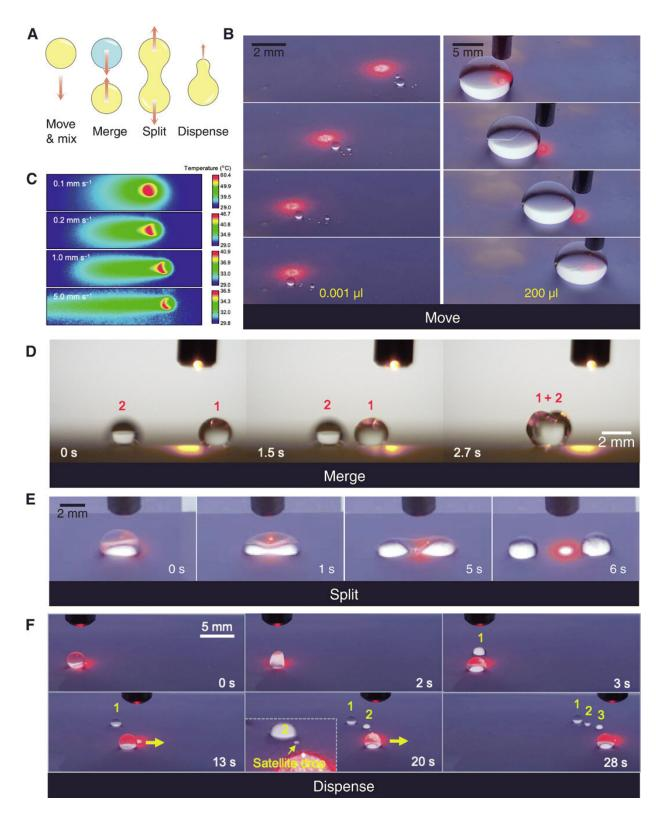
Fluidic operations. (A) Schematics showing four fundamental fluidic operations, including navigate, merge, split, and dispense. (B) Guided motions of a 0.001-µl
