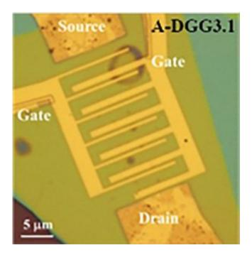
A scanning-electron microscopic top-view image of a fabricated graphene transistor structure under measurement. It features the unique transistor electrode structure called "double-grating gate," where two sets of gate electrodes that have a comb-like grating shape are prepared and arranged in an interdigitated fashion. Credit: Tohoku University
