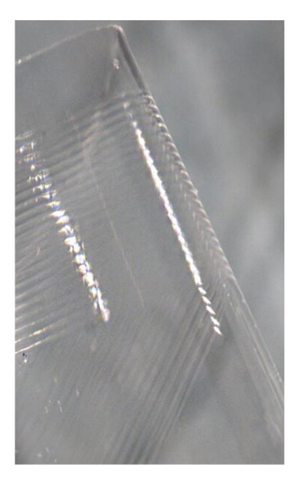
The waveguides are flexible and bend easily. Credit: College of Engineering
