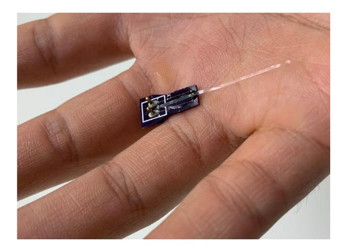
A Parylene photonic waveguide held in the palm for scale. Credit: Carnegie
