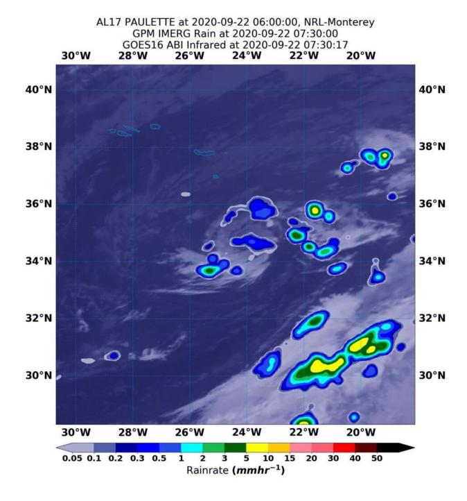
On Sept. 22 at 3:30 a.m. EDT (0730 UTC), NASA's IMERG estimated Tropical Storm Paulette was generating as much as (5 mm/0.20 inches of rain (yellow) around the center of circulation. The rainfall data was overlaid on infrared imagery from NOAA's GOES-16 satellite. Credit: NASA/NOAA/NRL
