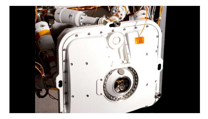
PIXL opens its dust cover during testing at NASA's Jet Propulsion Laboratory. One of seven instruments on NASA's Perseverance Mars rover, PIXL is located on the end of the rover's robotic arm. Credit: NASA/JPL-Caltech
