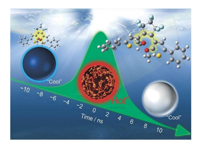
Schematic illustration of the heating of the nanoparticle and the amplification of the photochemical reaction during nanosecond laser pulse excitation. Intense nanosecond 532-nm pulse laser excitation to aqueous nanoparticles colloids of a photochromic diarylethene induced drastic amplification of the ring-opening reaction yield. This mechanism was explained as a 'photosynergetic response'
