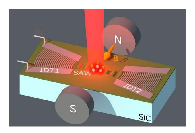
Surface acoustic waves (SAW) generated by radio-frequency signals applied to interdigital transducers (IDT) control the spin states of optically active color centers in SiC. The coupling strength depends on the spin projection direction of the color centers, which is controlled by an external magnetic field (B). Credit: A. Hernández-Mínguez
