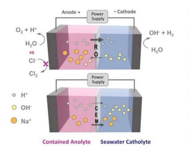
Here is a visual representation of how ion movement is affected by a reverse osmosis (RO) membrane versus a cation-exchange membrane. Chloride ions from the seawater are not able to pass through the RO membrane and oxidize
