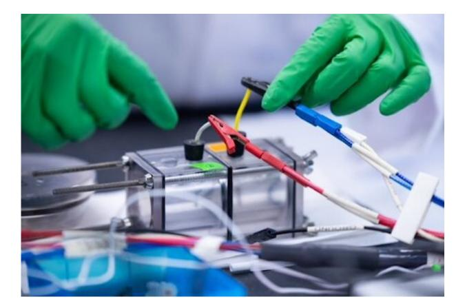
Sea water can be converted into hydrogen fuel using this design for a sea water electrolyzer, according to Penn State researchers. Credit: Tyler Henderson
